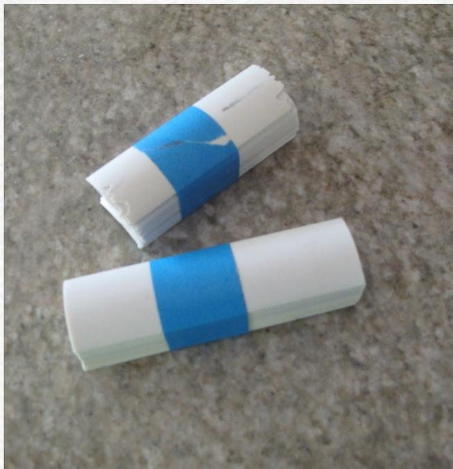
House Siding cut with tin snips or saw
